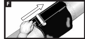
Gently heat the closure and pat it down with a gloved hand. Repeating this procedure, move from one side to the other. Smooth any wrinkles by gently working them outward from the centre of the closure with a roller.
